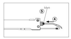
Place a new cartridge into the auto-feed iron (4).
