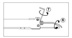
Align the cartridge tip with the guide nozzle (6) and tighten the cartridge screw (7).
