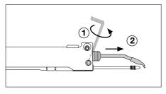
Loosen the cartridge screw (1) to release the cartridge (2).
