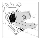
Remove the wiper by pulling it out.
