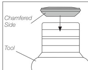
Push the sealing plug inside the tool.
