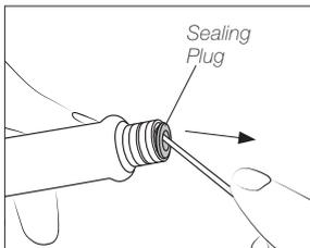
Introduce a small shaft or screwdriver, not deeper than 8 mm, lift and pull the sealing plug. Never use a cartridge to do this operation.
