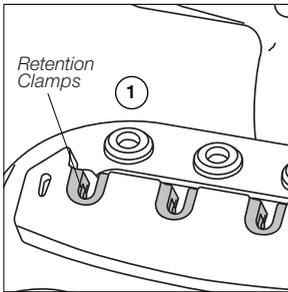
The cartridge extractor allows inserting / changing cartridges safely without switching off the tool. Cartridges are held in place thanks to the retention clamps (1).
