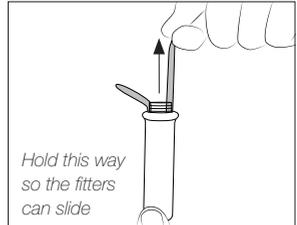
To remove the fitters, hold the grip and pull the fitters out. Use pliers if necessary.
