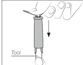
Push the grip with the fitters onto the tool.
