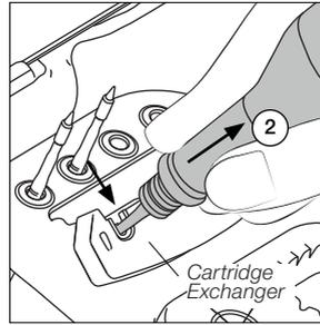
Place the tool with the cartridge over the cartridge exchanger slots and press down (1) until it clicks. To remove the cartridge pull out the tool (2).
