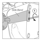
Loosen the screws (1) at the bottom.
