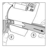
Hold the charging holder with one hand (2) and with the other pull the side band downward (3).
