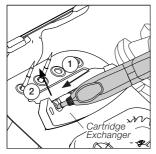
Place the tool over a cartridge and push the tool onto it to insert the cartridge (1). To release the tool with the cartridge inserted from the extractor, lift the tool upward (2).
