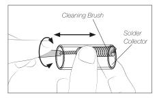
Introduce the cleaning brush into the empty solder collector and remove soldering residues with longitudinal and circular movements.
