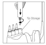
To remove the tip from the spanner, simply place the tip in one of the holes of the tip storage, screw it in lightly (only aprox. 1 turn) and pull the spanner out.
