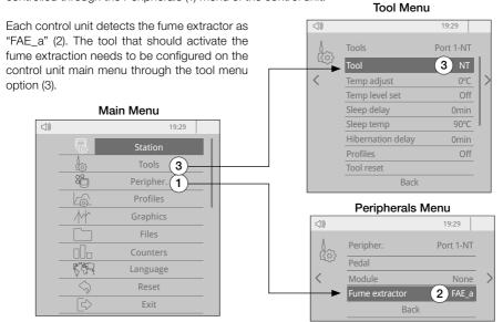
Connect up to 4 control units (connector FAE/ROBOT) to the fume extractor connectors (STATION 1, STATION 2, ...). Each tool connected to these control units can start and stop the fume extractor.
