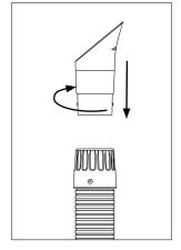
To install a new nozzle, turn the nozzle bayonet clockwise to lock it in place.
