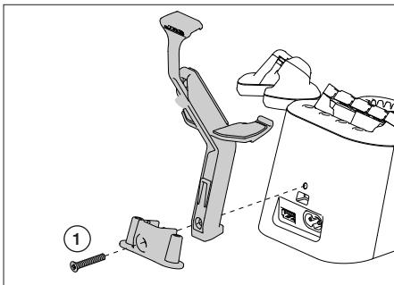
Align the display holder components as shown in the image and screw them to the charging base using the supplied DIN965 screw (1).
