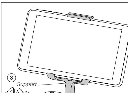
Place the display on the support (3). Adjust the height of the display holder tab and tighten the fixing knob.
