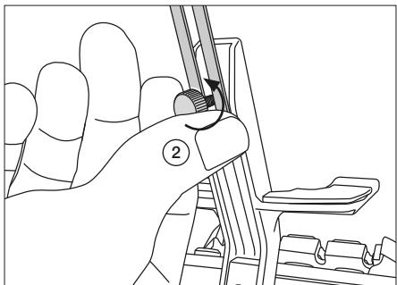
Loosen the fixing knob (2) enough so that the display holder tab can slide along the rear rail.
